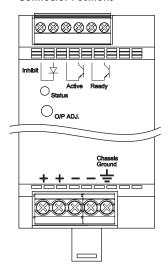
Max. terminal screw locked torque: 0.8 Nm
