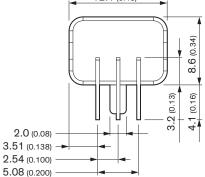
Dimensions in mm (inch) Tolerances: x.xx  $\pm 0.5$  ( $\pm 0.02$ ) Tolerances: x.xxx  $\pm 0.25$  ( $\pm 0.01$ ) Pin pitch tolerances:  $\pm 0.10$  ( $\pm 0.04$ )
