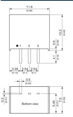
Dimensions in mm (inch) Tolerances: x.x  $\pm 0.5 (\pm 0.02)$ x.xx  $\pm 0.25 (\pm 0.01)$ Pin dimension tolerance:  $\pm 0.1 (\pm 0.04)$
