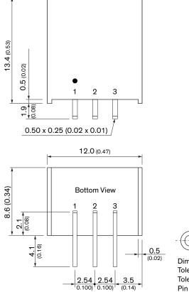
Dimensions in mm (inch) Tolerances: x.xx  $\pm 0.5$  ( $\pm 0.02$ ) Tolerances: x.xxx  $\pm 0.25$  ( $\pm 0.01$ ) Pin dimension tolerances:  $\pm 0.10$  ( $\pm 0.04$ )
