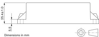
Max. mounting screw tightening torque: 0.29±0.049 Nm (3±0.5 kgfcm)
