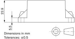
Mounting screw locked torque: 0.29 Nm (3 kgfcm)
