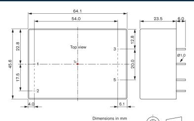
Tolerances ±0.5 mm Pin tolerances ±0.1 mm
