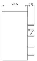
Dimensions in mm Tolerances ±0.5 mm Pin tolerances ±0.1 mm
