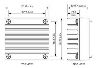
$\begin{array}{ll} \mbox{Dimensions in mm (inch)} \\ \mbox{Tolerances: } x.x & \pm 0.5 \ (x.xx \pm 0.02) \\ & x.xx & \pm 0.25 \ (x.xxx \pm 0.01) \end{array}$
