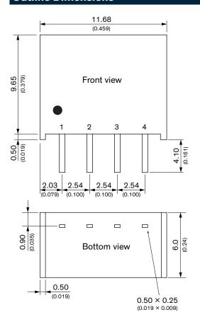
Dimensions in mm (inch) Tolerances: x.x  $\pm$ 0.5 (x.xx  $\pm$ 0.02) x.xx  $\pm$ 0.25 (x.xxx  $\pm$ 0.01) Pin dimension tolerance:  $\pm$ 0.1 ( $\pm$ 0.004)
