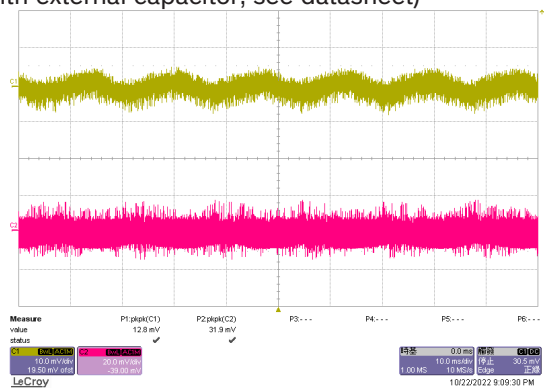
Typical Output Ripple and Noise at 230 Vin Out 1: 5V/7.6A, Out 2: 24V/1.75A (with external capacitor; see datasheet)
