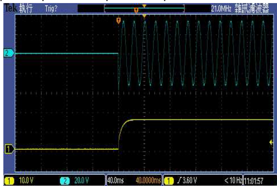
Typical Input Start-Up and Output Rise Characteristic
