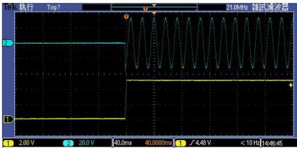
Typical Input Start-Up and Output Rise Characteristic
