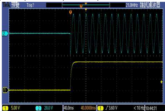
Typical Input Start-Up and Output Rise Characteristic
