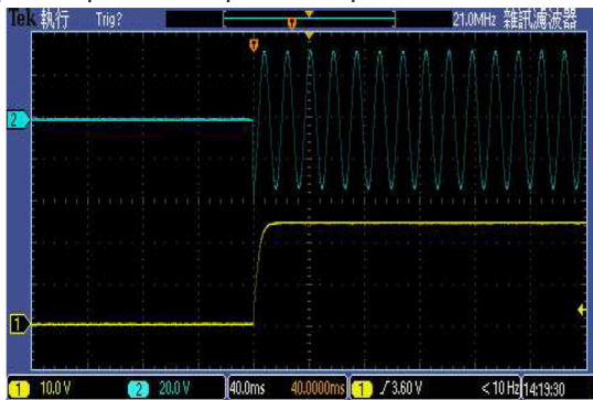
Typical Input Start-Up and Output Rise Characteristic
