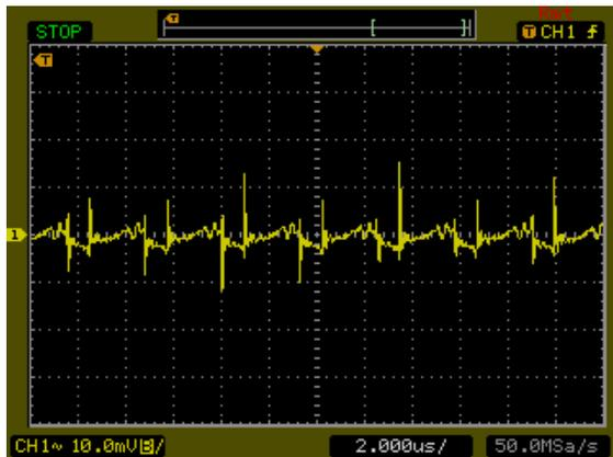
Typical Output Ripple and Noise.
