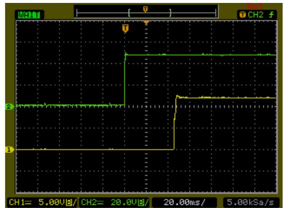
Typical Input Start-Up and Output Rise Characteristic
