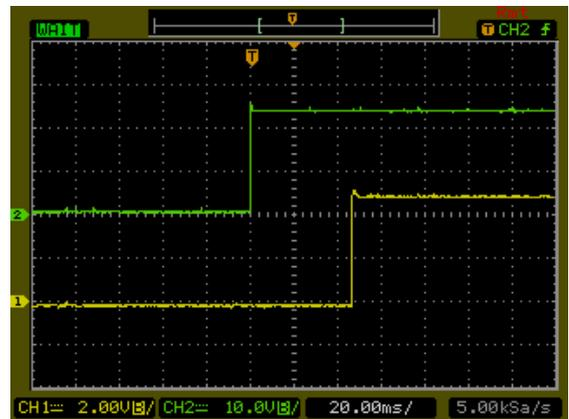
Typical Input Start-Up and Output Rise Characteristic
