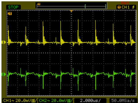
Typical Output Ripple and Noise.
