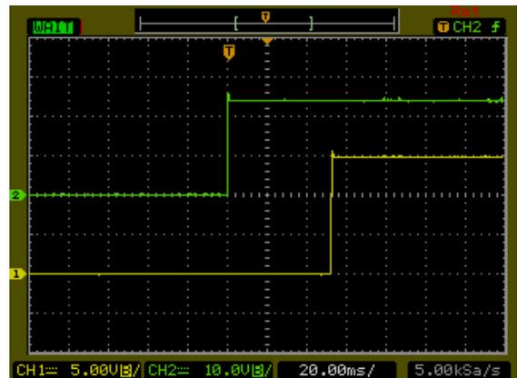
Typical Input Start-Up and Output Rise Characteristic
