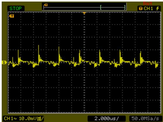
Typical Output Ripple and Noise.
