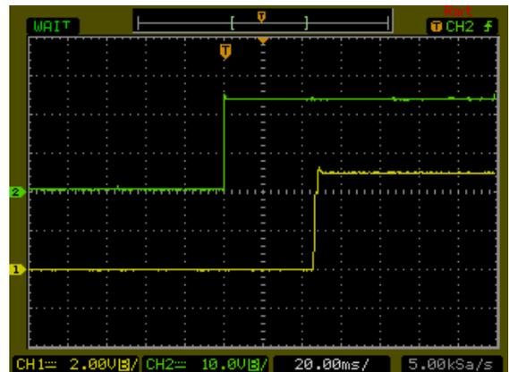
Typical Input Start-Up and Output Rise Characteristic
