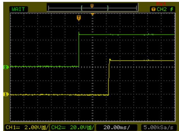
Typical Input Start-Up and Output Rise Characteristic
