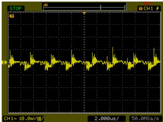
Typical Output Ripple and Noise.
