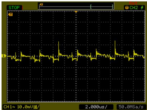
Typical Output Ripple and Noise.
