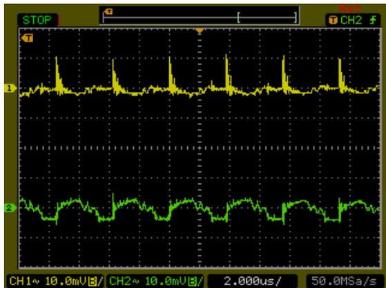
Typical Output Ripple and Noise.
