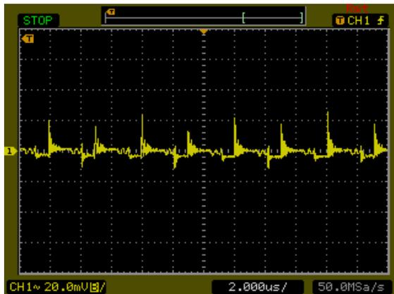
Typical Output Ripple and Noise.
