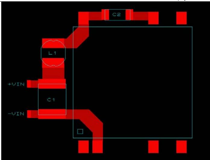
Recommended PCB Layout with Input Filter
