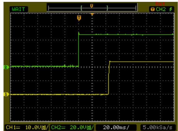
Typical Input Start-Up and Output Rise Characteristic
