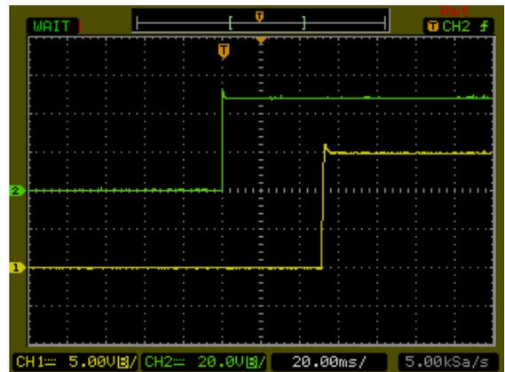
Typical Input Start-Up and Output Rise Characteristic
