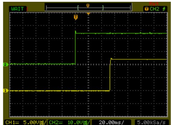
Typical Input Start-Up and Output Rise Characteristic
