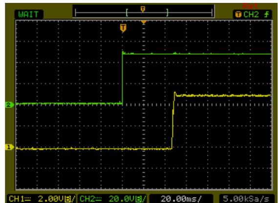
Typical Input Start-Up and Output Rise Characteristic
