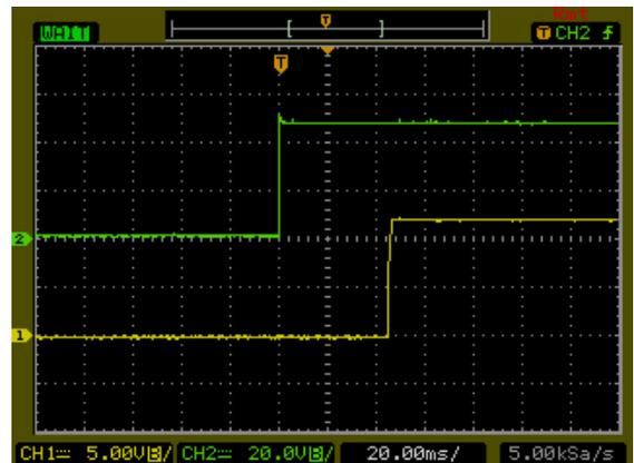
Typical Input Start-Up and Output Rise Characteristic
