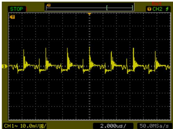
Typical Output Ripple and Noise.
