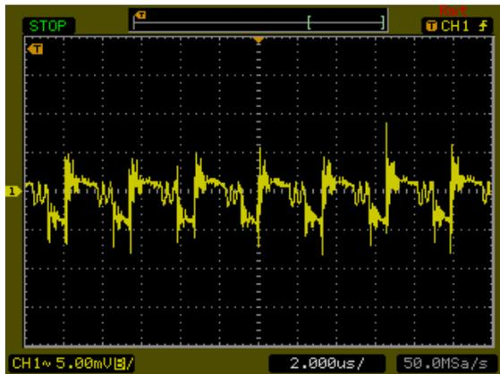
Typical Output Ripple and Noise.
