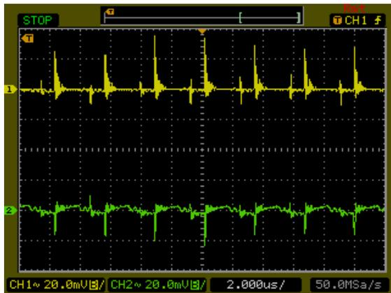
Typical Output Ripple and Noise.
