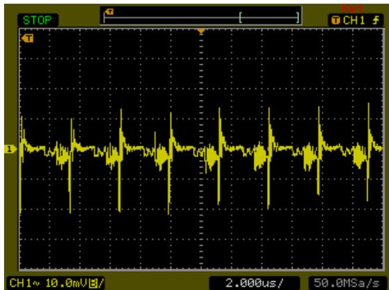
Typical Output Ripple and Noise.
