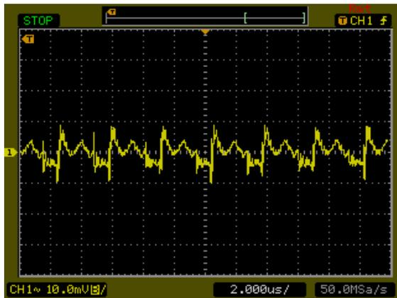
Typical Output Ripple and Noise.
