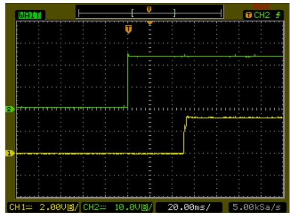
Typical Input Start-Up and Output Rise Characteristic
