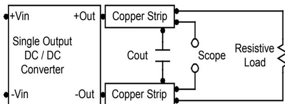
**Output voltage and efficiency measurement test up**
