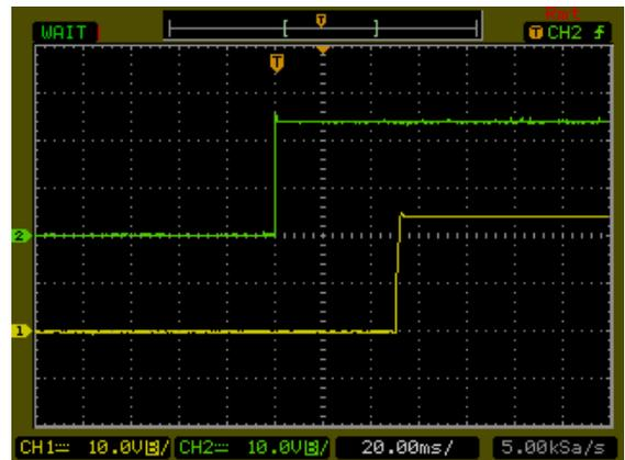
Typical Input Start-Up and Output Rise Characteristic
