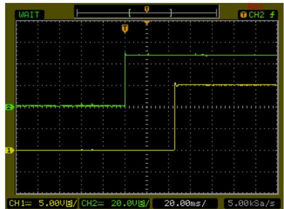
Typical Input Start-Up and Output Rise Characteristic
