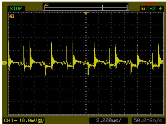
Typical Output Ripple and Noise.
