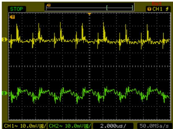
Typical Output Ripple and Noise.
