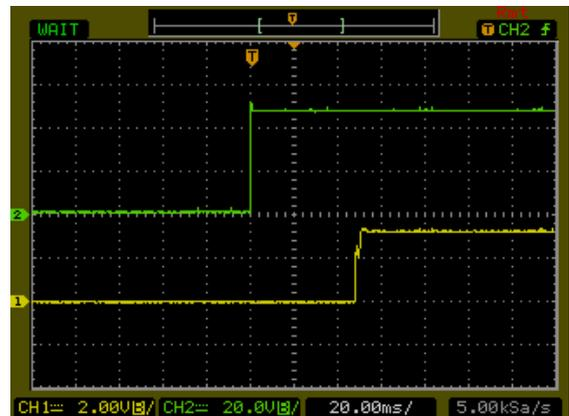
Typical Input Start-Up and Output Rise Characteristic
