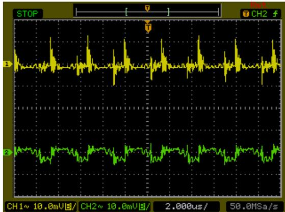
Typical Output Ripple and Noise.
