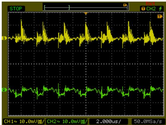
Typical Output Ripple and Noise.
