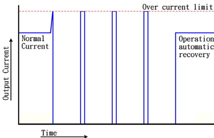
Hiccup operation has none of the drawbacks of the other two protection methods, although its circuit is more complicated because it requires a timing circuit. The excess heat due to overload lasts for only a short duration in the hiccup cycle, hence the junction temperature of the power devices is much lower.
