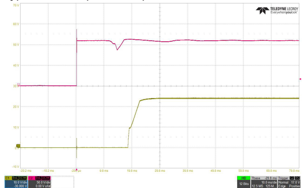
Typical Start-Up and Output Rise Characteristic
