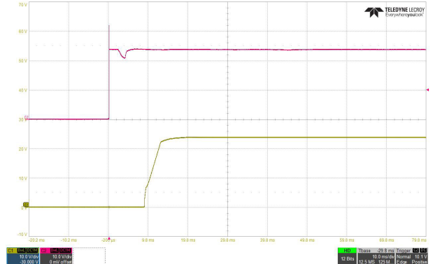
Typical Start-Up and Output Rise Characteristic
