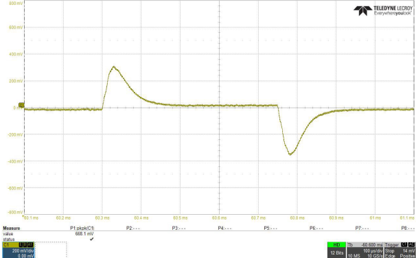
Transient Response to Dynamic Load Change (25%)
