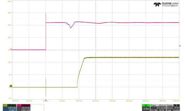
Typical Start-Up and Output Rise Characteristic
