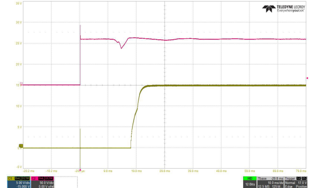
Typical Start-Up and Output Rise Characteristic
