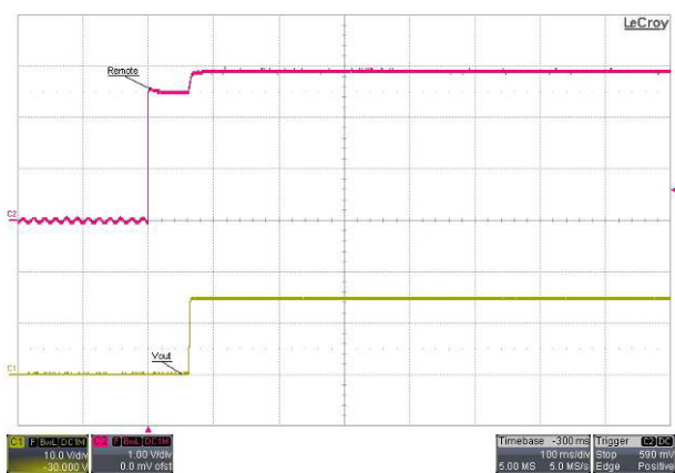
ON/OFF Voltage Start-Up and Output Rise Characteristic V_{in} = V_{in\ nom} ; Full Load
