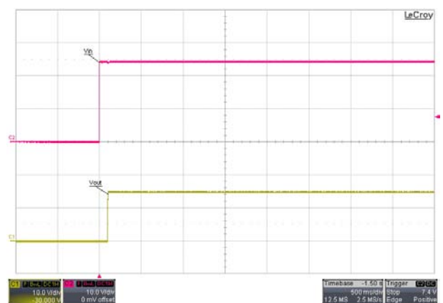
Typical Input Start-Up and Output Rise Characteristic
