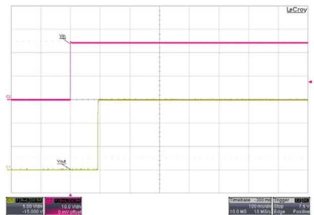
Typical Input Start-Up and Output Rise Characteristic V_{in} = V_{in\ nom} ; Full Load
