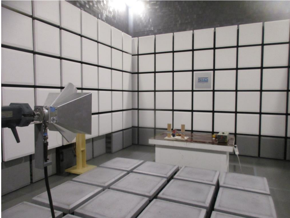
Figure 3: Radiated electromagnetic field immunity test
