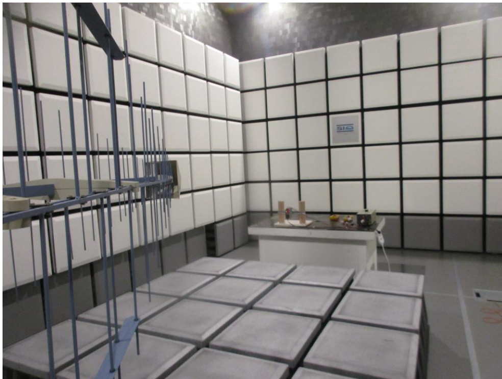
Figure 2: Radiated electromagnetic field immunity test
