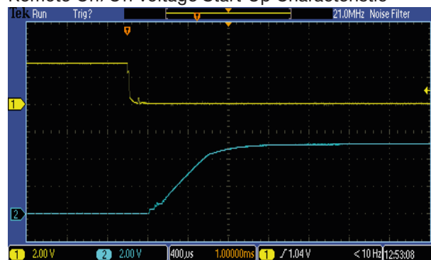
Remote On/Off Voltage Start-Up Characteristic
