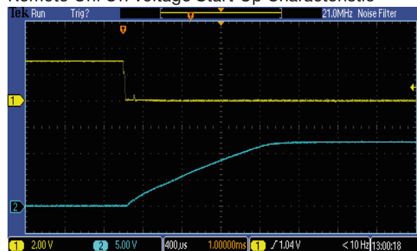
Remote On/Off Voltage Start-Up Characteristic
