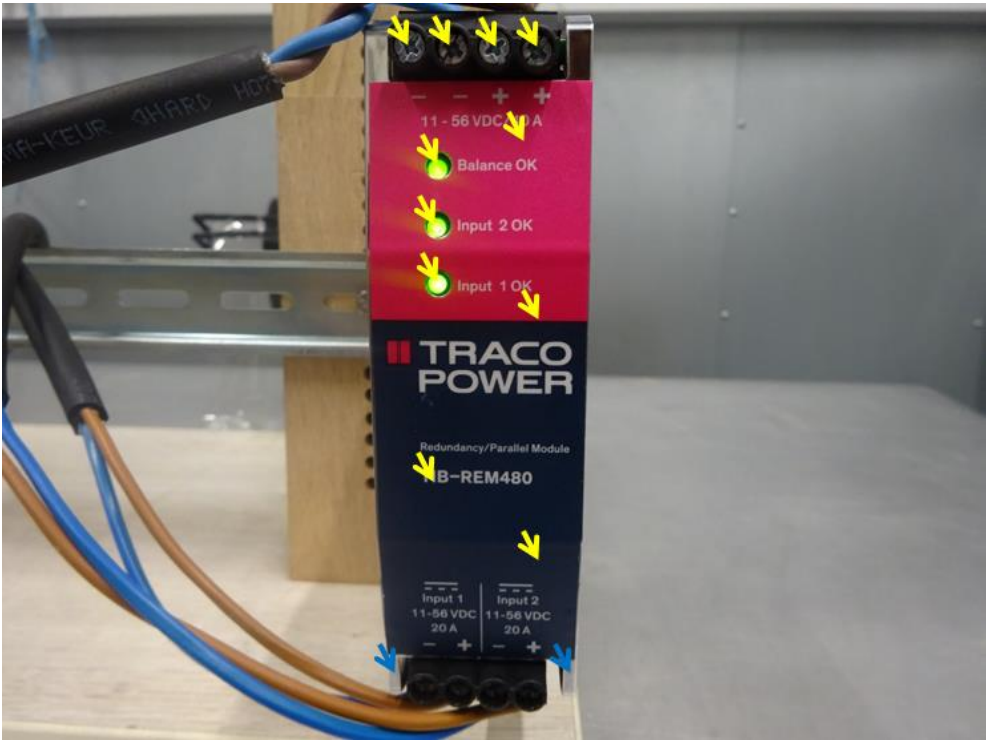
Figure 1: Electrostatic discharge immunity measurement
