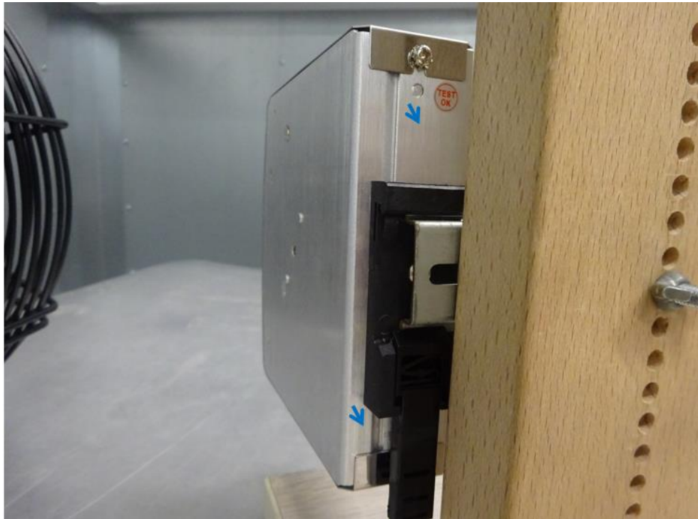
Figure 6: Electrostatic discharge immunity measurement
