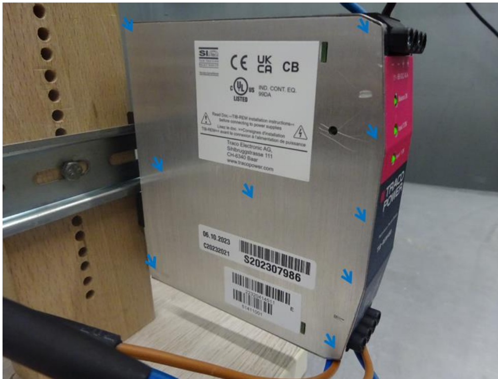
Figure 4: Electrostatic discharge immunity measurement
