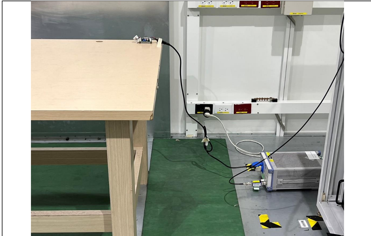
Conducted Disturbance: Mode 1, LISN
