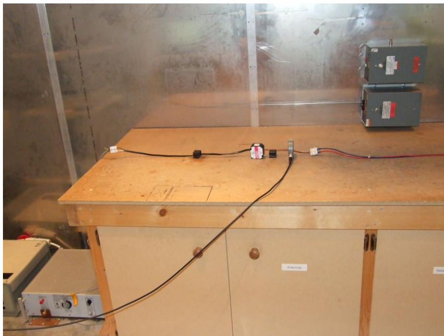
Figure 1. Test set-up for measurement of disturbance power similar to IEC61204-3
