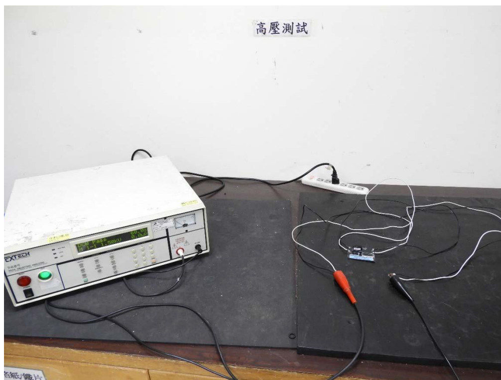
Voltage withstand test
