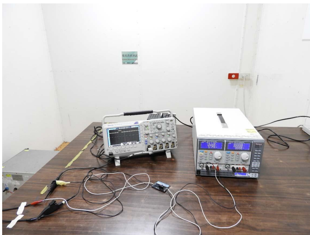
Supply variation Test (Test Voltage: 154.0Vdc)
