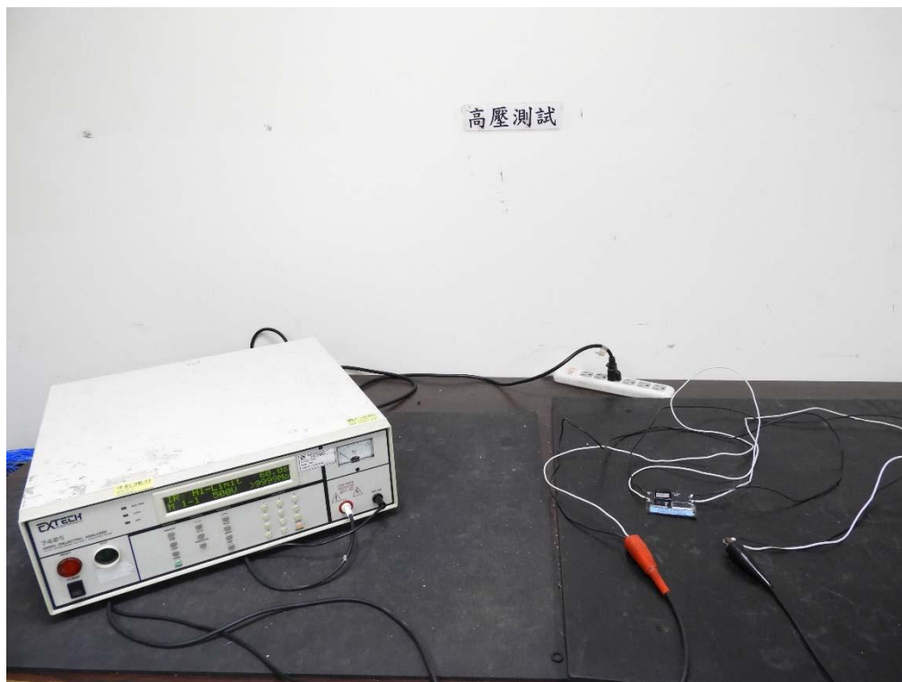
Insulation measurement test (before voltage withstand test)
