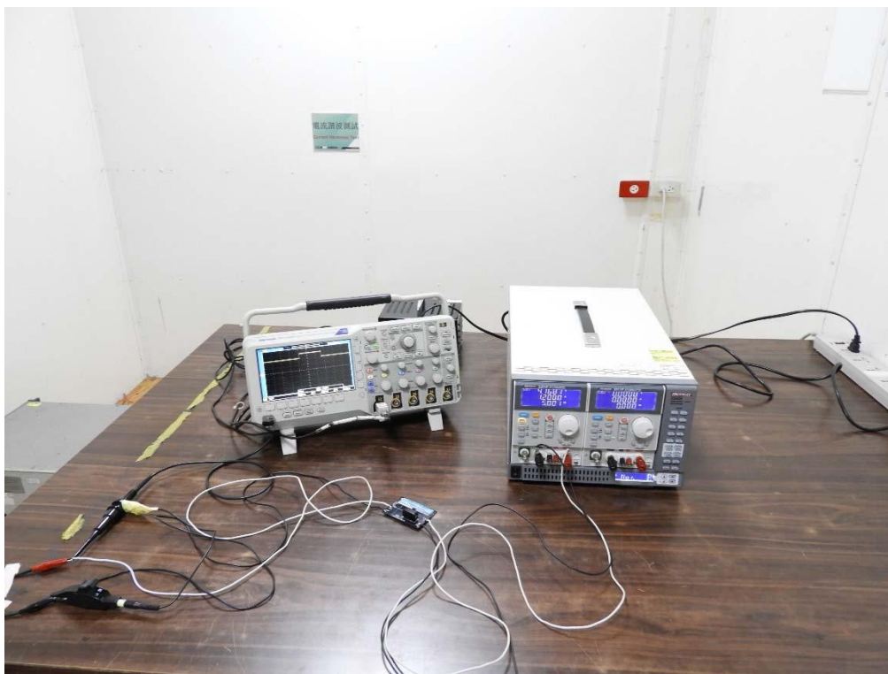
Supply variation Test (Test Voltage: 154.0Vdc)
