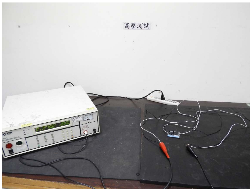
Insulation measurement test (after voltage withstand test)
