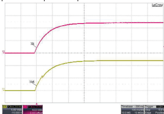
Load Variation versus Output Voltage
