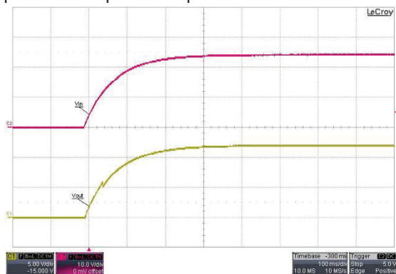
Load Variation versus Output Voltage
