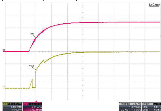
Load Variation versus Output Voltage
