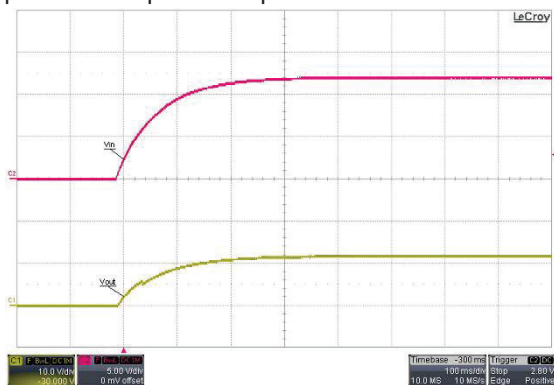
Load Variation versus Output Voltage
