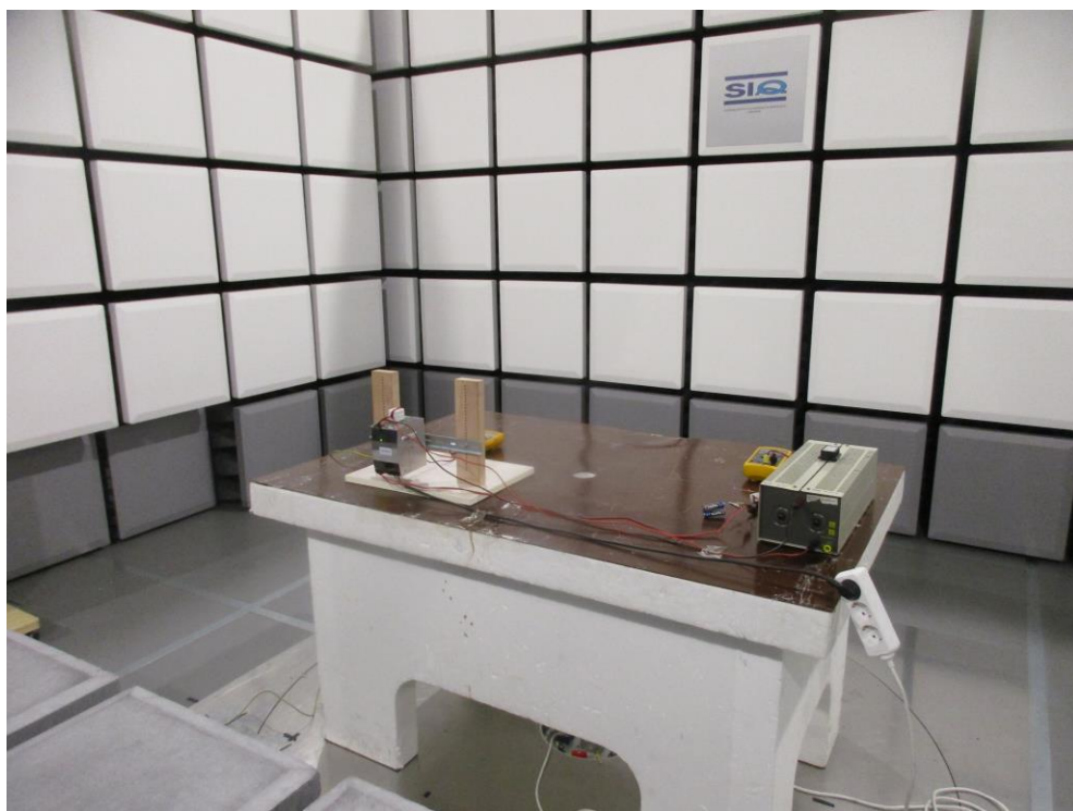
Figure 4: Radiated electromagnetic field immunity test
