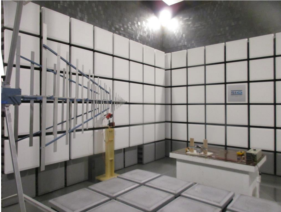
Figure 1: Radiated electromagnetic field immunity test
