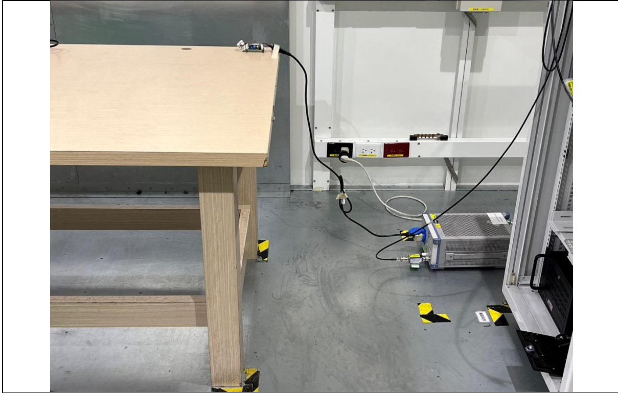
Conducted Disturbance: Mode 1, LISN
