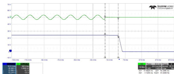
Typical Hold-Up Characteristic at 115 Vin
