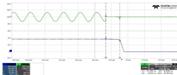
Typical Hold-Up Characteristic at 230 Vin
