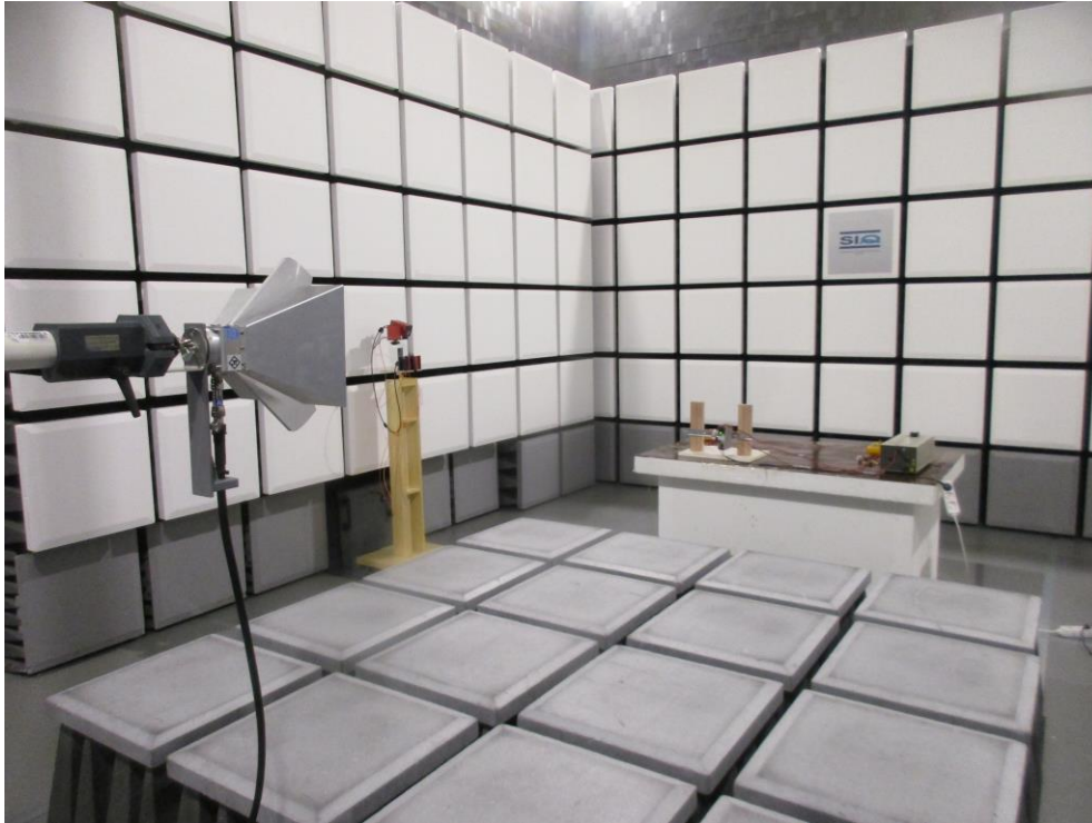
Figure 3: Radiated electromagnetic field immunity test
