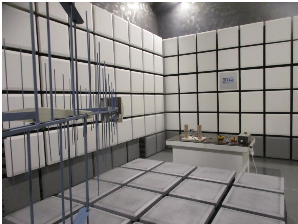
Figure 2: Radiated electromagnetic field immunity test
