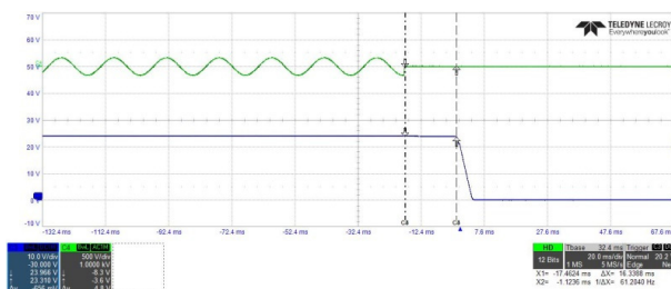
Typical Hold-Up Characteristic at 115 Vin
