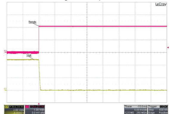
Remote on/off Voltage Start-Up Characteristic
