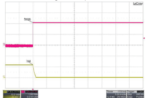
Remote on/off Voltage Start-Up Characteristic
