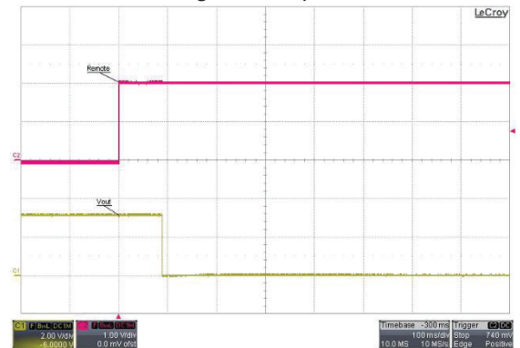
Remote on/off Voltage Start-Up Characteristic
