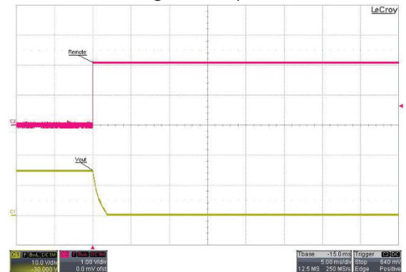
Remote on/off Voltage Start-Up Characteristic
