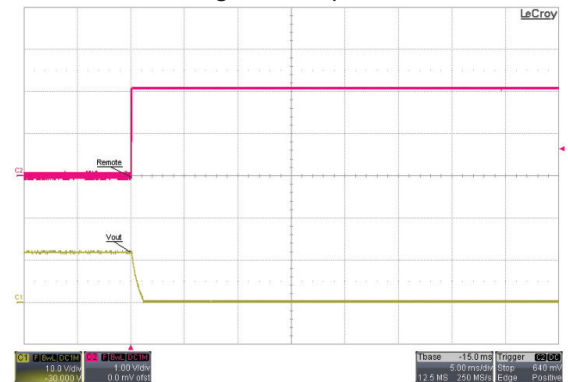
Remote on/off Voltage Start-Up Characteristic
