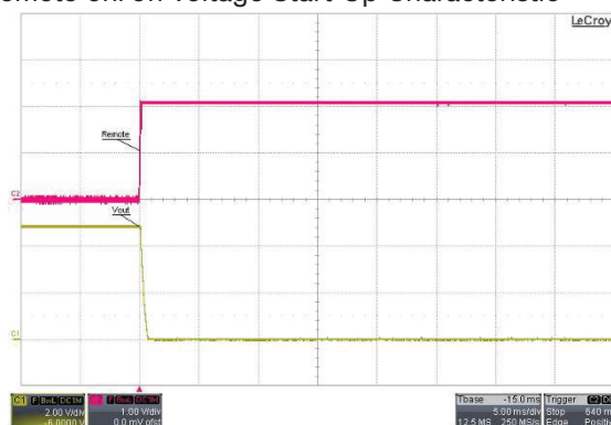
Remote on/off Voltage Start-Up Characteristic
