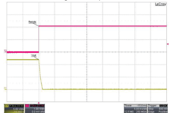
Remote on/off Voltage Start-Up Characteristic
